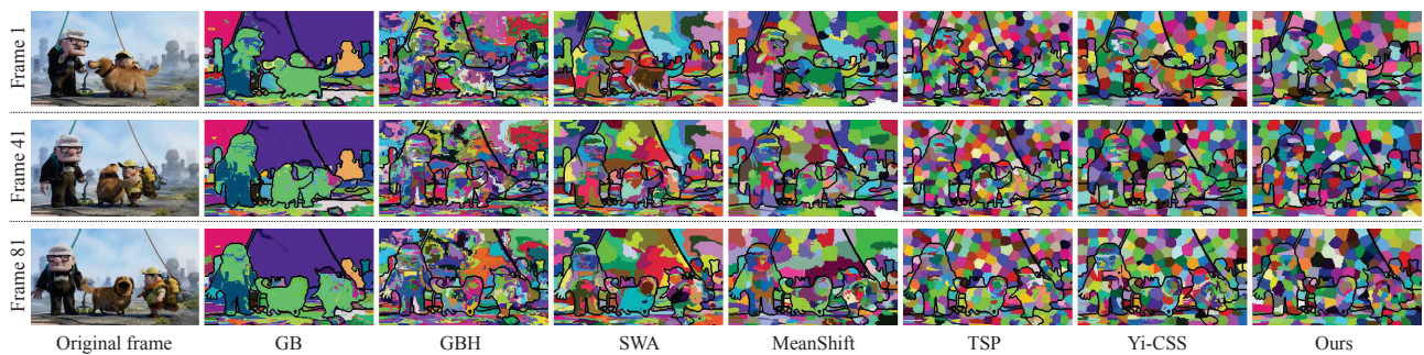
Figure 2. Visual comparison of supervoxels (which have different colors and are clipped on each image frame) computed by GB [14], GBH [17], SWA [32, 33, 10], MeanShift [29], TSP [7], Yi-CSS [46] and our method. All the methods generate approximately 1,000 supervoxels. Our method produces better results than the other methods in terms of UE3D, BRD, SA3D and CO on four video datasets (Figure 8).
